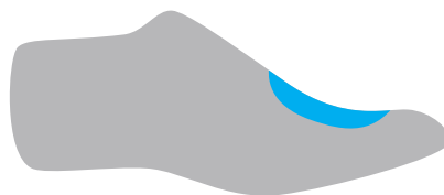
B B lasts are shallower at the forefoot - forefoot being from the joint forwards
